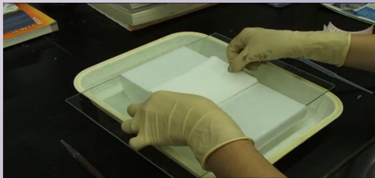
Cover with 2 sheets of wet Whatman 3MM filter paper
